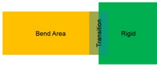
Transition zone must overlap bend area by 15 mils.
